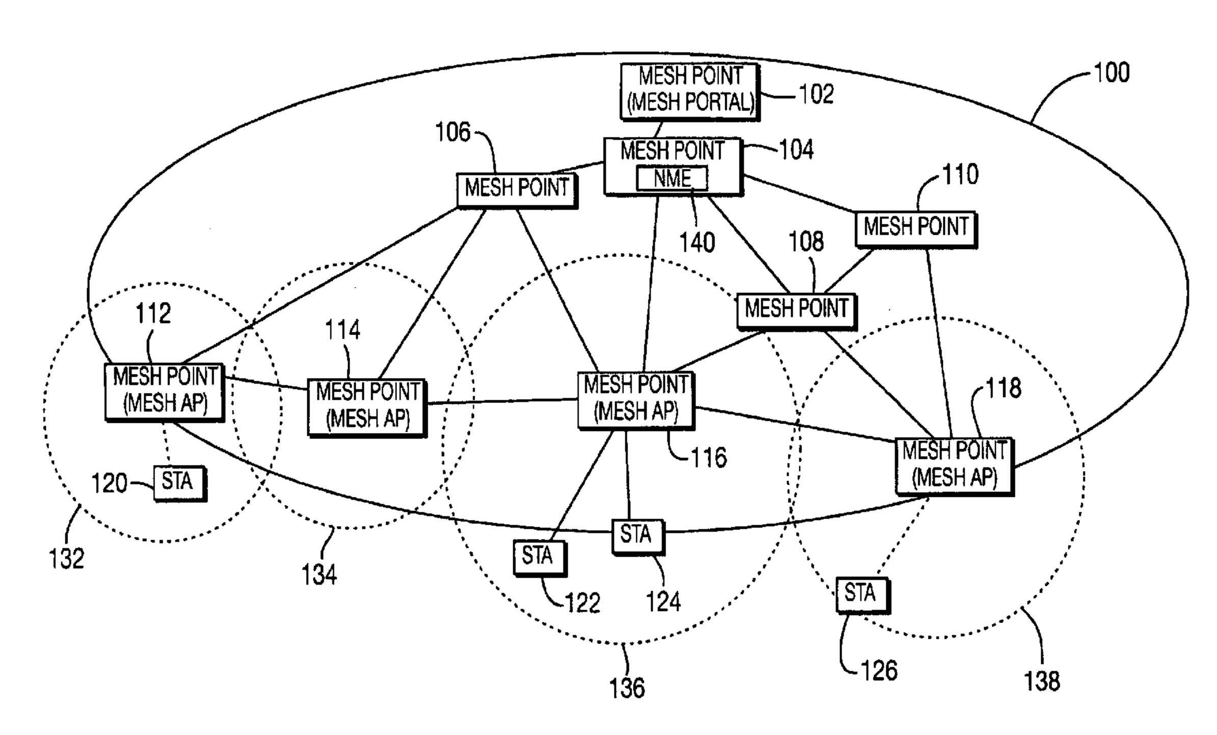
(57) Abstract: High throughput channel operation in a mesh wireless local area network (WLAN) is disclosed. A mesh network comprises a plurality of mesh points and a network management entity (NME). The NME is configured to retrieve capability and configuration data from the mesh points. The NME configures at least one mesh point with respect to IEEE 802.11n channelization and legacy protection mode based on the capability and configuration data.
