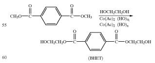
1.4 moles of dimethyl terephthalate (277 g) and 7.2 moles of ethylene glycol (445 g) were weighed into a one-liter round-bottomed flask connected to a vacuum line. A catalytic amount of cobalt (II) acetate tetrahydrate (180 mg, 0.5 mole) and calcium acetate hydrate (90 mg, 0.4 mole) were
