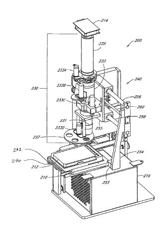
(57) Abstract: An imaging system (200) for automation of sample monitoring includes an image capture device (214) that cooperates with a lens assembly (230) for imaging the samples on a sample plate (212) on a sample plate mount (210) the lens assembly (230) and another translator positions the sample plate (210) for acquisition of the images. Some embodiments of the system include a light source (216) configured to provide low temperature, flash illumination of a sample plate.
