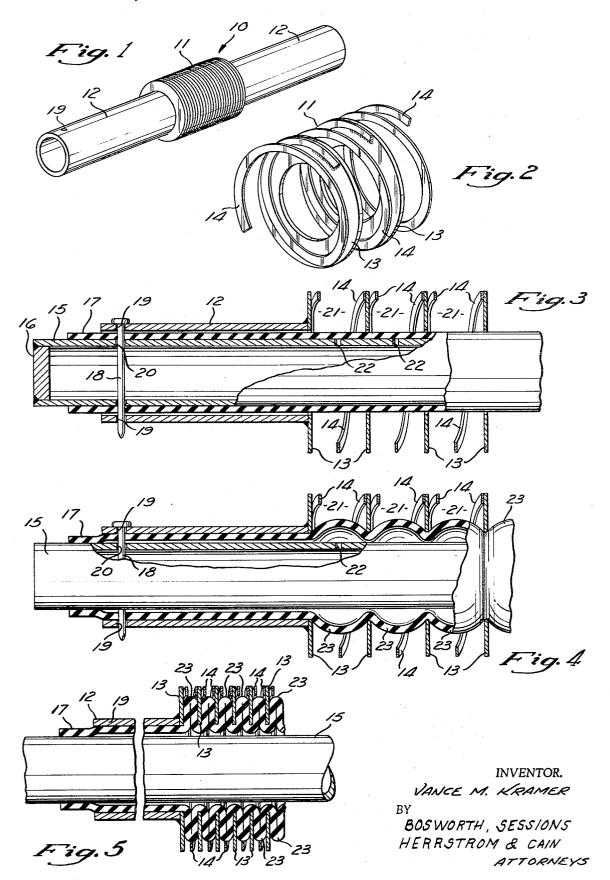
APPARATUS FOR MAKING FLEXIBLE TUBING WITH ANNULAR CORRUGATIONS
