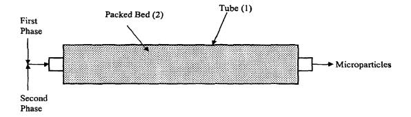
Figure 2 – A Typical Packed Bed Emulsification System
