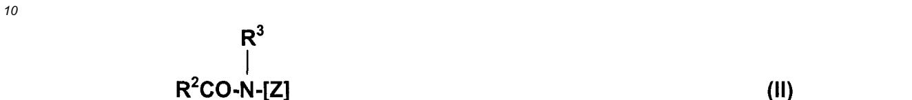
where R<sup>2</sup>CO is an aliphatic acyl group containing 6 to 22 carbon atoms, R<sup>3</sup> is hydrogen, an alkyl or hydroxyalkyl group containing 1 to 4 carbon atoms and [Z] is a linear or branched polyhydroxyalkyl group containing 3 to 12 carbon atoms and 3 to 10 hydroxyl groups.
