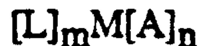
15 where L is a bulky ligand: A is leaving group and or a ligand bonded to M and capable of inserting an olefin between the M-A bond, M is a transition metal and m and n are such that the total ligand valency corresponds to the transition metal valency. Preferably the catalyst is four co-ordinate such that the compound is ionizable to a  $1^+$  charge state.
