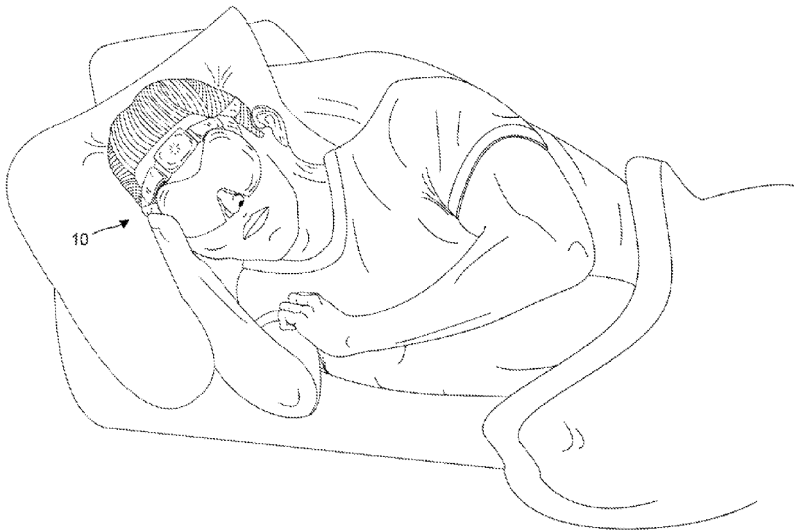
HEADBAND AND EYE MASK SECURE SENSORS TO FOREHEAD DURING SLEEP
