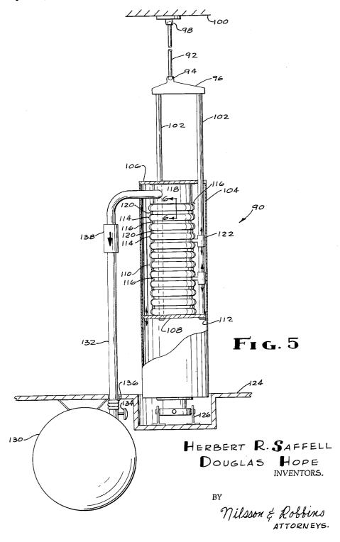
3,233,886 PNEUMATIC SHOCK ISOLATOR AND METHOD Herbert R. Saffell, El Segundo, and Douglas Hope, Seal Beach, Calif. Filed Apr. 9, 1963, Ser. No. 271,675 4 Claims. (Cl. 267—1)
