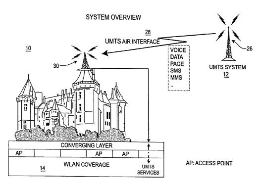
(57) Abstract: A method enabling a wireless remote terminal (UE) to access a universal mobile telecommunication system (UMTS) through a wireless local area network (WLAN) wherein UMTS services are transmitted to a format converter from a UMTS transceiver and the format converter changes the format of received messages to a WLAN format before transmission to the UE which is operating in the WLAN mode.
