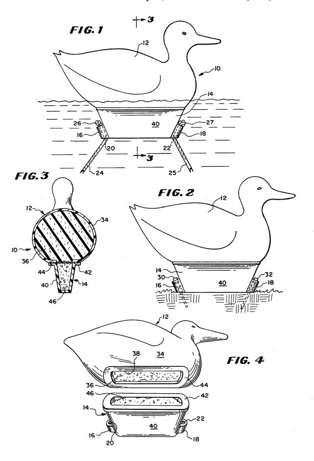
receiving stakes for securing the goose decoy in position on the ground.
