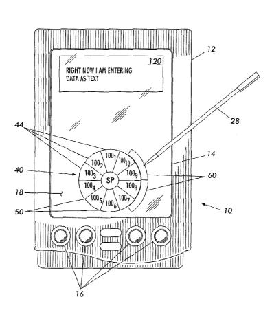
(57) Abstract: The invention is a method and apparatus for entry of alphanumeric characters or symbols, employing fewer data entry keys than the number of characters to be selected from. In particular the invention "multiplexes" a given display area (14) to control the display of specific character groupings (44) and to facilitate user selection and entry or editing of characters.
