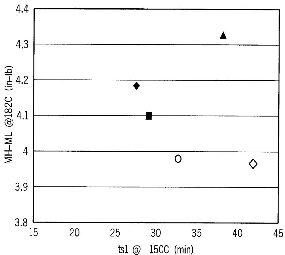
The legend is enclosed in a rectangular box. It lists five entries, each consisting of a symbol and text: a diamond for '1.8% VCP', a square for '1.8% VCP + 0.25% Allyl-TEMPO', a triangle for '1.8% VCP + 0.54% Stearyl-U-TEMPO', a circle for '1.8% VCP + 0.20% Amino-TEMPO', and an open diamond for '1.8% VCP + 0.40% 4-Hydroxy-TEMPO'.
