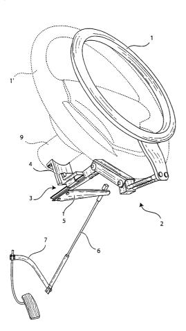
(57) Abstract: The invention relates to device for manual acceleration providing a transmission of the acceleration force acting outside the steering wheel (11) operating range.
