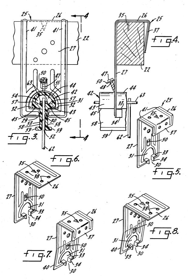
FIG. 5 is an isometric view of the beam hanger clip shown in FIGS. 3 and 4.
