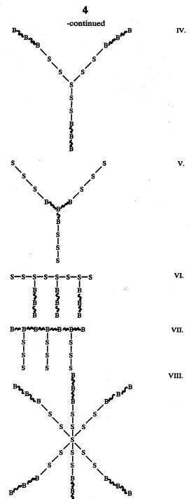
The polymer skeleton is modified to the cationic hydrophilic-hydrophobic block or graft copolymer through hydrogenation of the polybutadiene segments followed by chemical modification of the polystyrene segments to strong polyelectrolytes with cationic sites fixed onto the polymer backbone.
