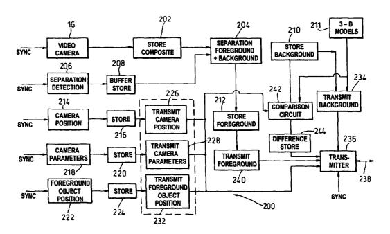
(57) Abstract: A narrow bandwidth broadcasting system for transmission of video and television via low bandwidth medium such as internet or radio links.
