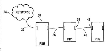
(57) Abstract: A method and apparatus for managing an Inline Power relationship between and among a first network device acting as power sourcing equipment (PSE) to provide Inline Power to a second Powered Device (PD) and a third device. In one aspect of the invention, the powered device(s) and the third device are powered (at least in part) by the PSE using inline power from at least one port (which may include more than one PSE) and they are powered over one or more sets of cables.
