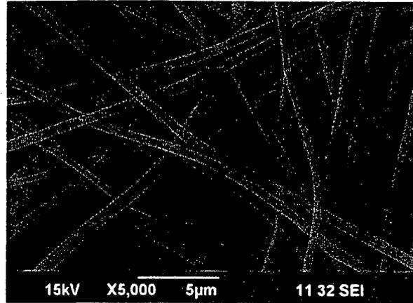
Figure 4: SEM image showing microscopic fiber morphology of TMZ and O6-BG co-loaded PLA-PLGA/PLGA wafer.
