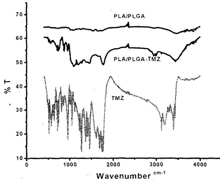
Figure 6: FTIR results showing interaction of TMZ with PLA-PLGA blend polymeric matrix
