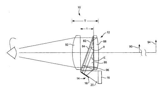
(57) Abstract: A virtual image display system is provided which comprises a non-emissive, reflective microdisplay (18) which forms a source object; an optical system which forms a magnified, virtual image of the source object from light reflected off the microdisplay; a light source system (16) which produces light to illuminate the display system; and an illumination system which forms at least two virtual light sources to illuminate the display system.
