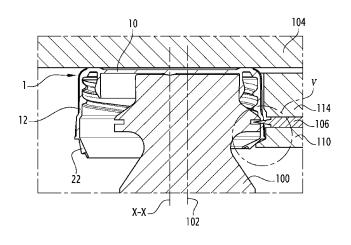
thereby pass from a molding configuration to an intermediate prefolded configuration. The retention strip is then folded until it passes into an operating configuration. In some implementations, the folding of the retention strip may pass the retention strip from an intermediate prefolded configuration to an operating configuration.
