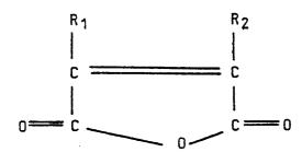
wherein  $R_1$  and  $R_2$  are hydrogen or a halogen. Suitable examples additionally include chloro-maleic anhydride, itaconic anhydride, hemic anhydride or the corresponding dicarboxylic acids, such as maleic acid or fumaric acid or their monoesters, etc.
