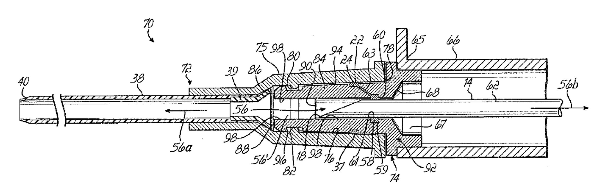
(57) Abstract: A generally rigid molded plastic catheter hub attachment (16, 52, 74) includes one or more co-molded elastomeric gaskets (22, 58).
