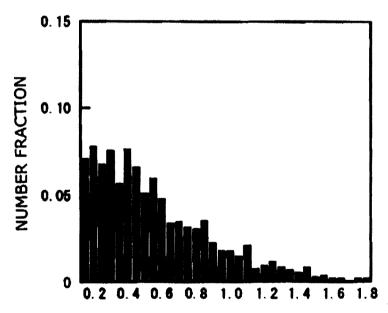
GRAIN SIZE OF RETAINED AUSTENITE GRAIN ( $\mu m$ )
