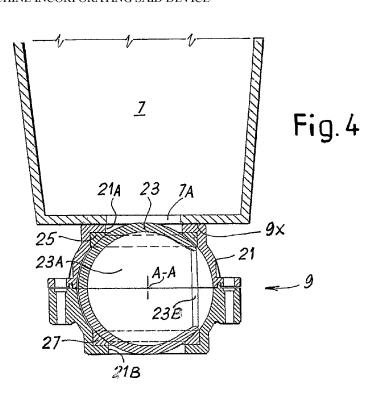
(57) Abstract: The device (9) comprises a dosing element (23) housed in a housing seat (21) equipped with an inlet (21A) for feed of the food product and with an outlet (21 B) for dispensing the food product. The dosing element rotates in the housing seat and has a hollow body with an opening (23B) for feed and delivery of the food product. With rotation of the dosing element the hollow body can be taken into alignment alternatively with the inlet or with the outlet of the housing seat (21).
