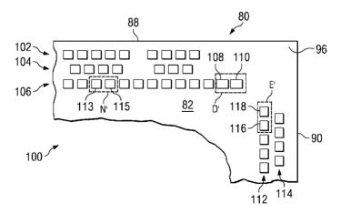
(57) Abstract: A bonded structure formed by connecting an electrical member to a substrate. A plurality of conductive bumps is located on the electrical member surface and a plurality of contact pads is located on a substrate. At least one of the conductive pads aligned with a non-planar area of the electrical member or substrate and having a surface area larger than a contact pad located outside the non-planar area. The conductive bumps are joined with the conductive pads.
