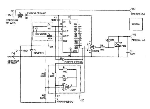
(57) **Abstract:** A heating device and method for de-icing or de-fogging the surface of a vehicle mirror. The device is activated upon ignition of the vehicle engine, and remains activated for a predetermined period of time. During the vehicle's journey the heater may be re-activated if the temperature of the mirror surface falls below a pre-set minimum threshold.
