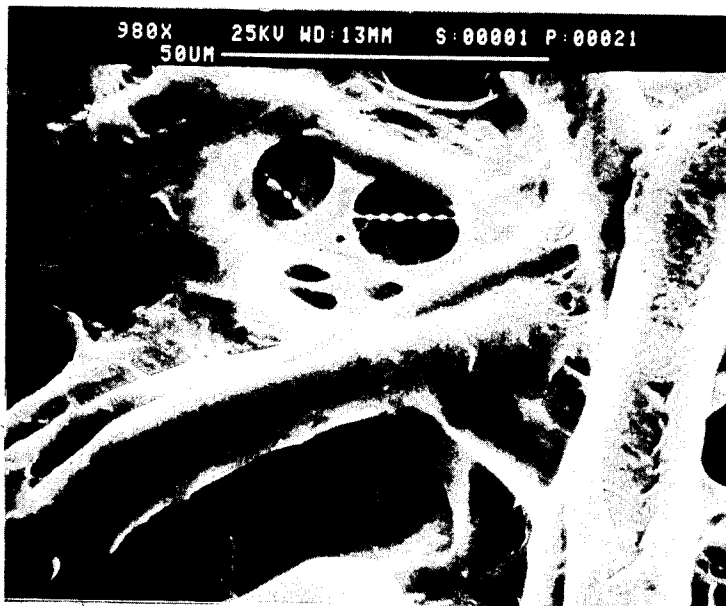
PURE COTTON SUBSTRATE TREATED WITH ETHYL ACRYLATE, 30% MONOMER ADDITION
