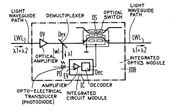
LIGHT WAVEGUIDE TELECOMMUNICATION SYSTEM HAVING ONE OR MORE OPTICAL SWITCHES LYING IN THE LIGHT WAVEGUIDE **PATH**
