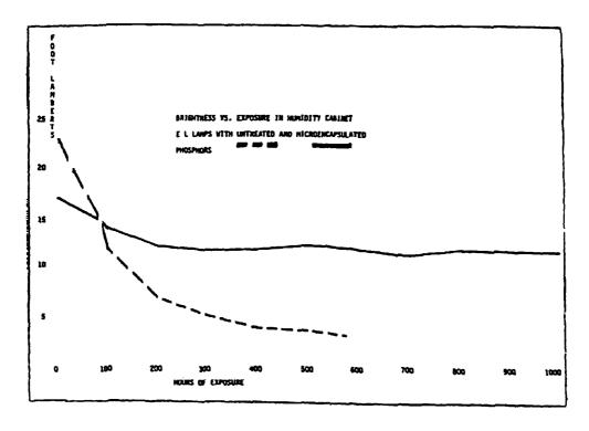
**(57) Abstract:** Microencapsulated particles having improved resistance to moisture and extended release capabilities are produced by microencapsulating the particles in a film-forming, cross-linked, hydrolyzed polymer.
