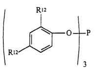
wherein each R<sup>12</sup> is the same or different alkyl, preferably alkyl of 3 to 7 carbons, and more preferably tertiary butyl. Substituted triazines useful in the present invention useful as an ultraviolet light absorber (UV absorbent) have a melting point of at least 140°C, preferably at least 144°C, and more preferably at least 148°C. Preferred substituted triazines have the formula
