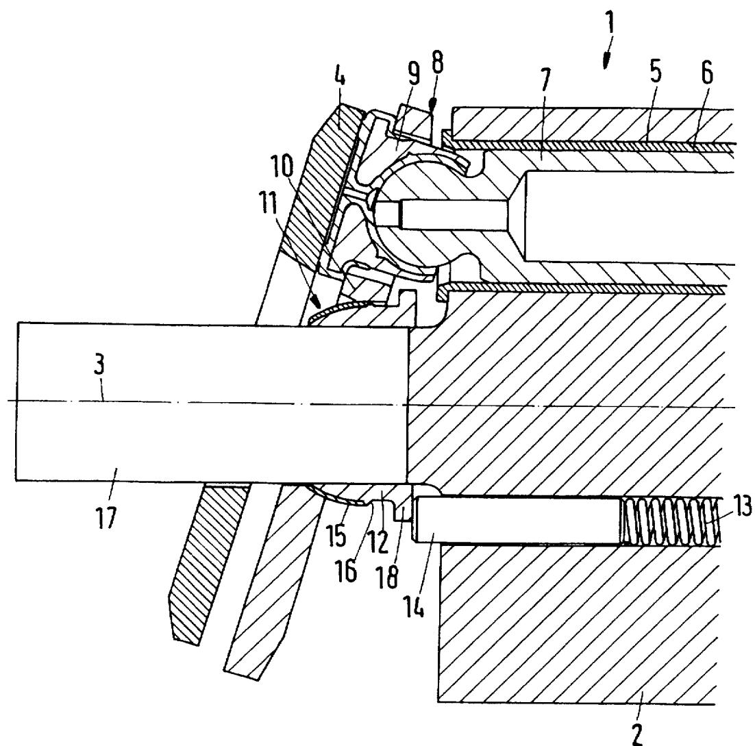
**HYDRAULIC AXIAL PISTON MACHINE****BACKGROUND OF THE INVENTION**
