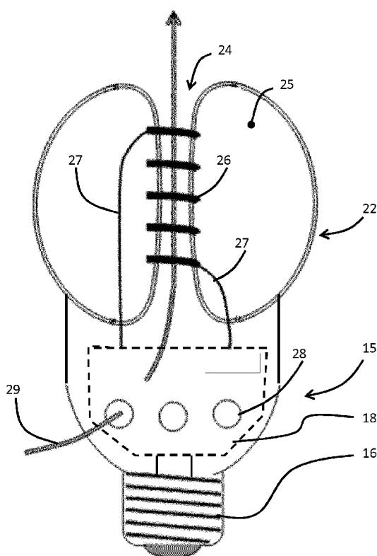
(57) Abstract: An LED light bulb has a light emitting bulb part 22 which comprises a central core 24 running from the top towards the bottom and which provides an open passageway at least at the top. The LEDs are mounted in thermal contact around the central core 24. This design provides an air flow to promote cooling of the LEDs. This in turn enables a reduced size and cost of the heat sink, or avoids the need for a heat sink altogether.
