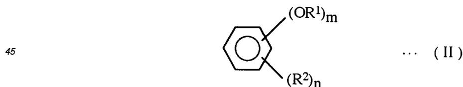
wherein  $\text{R}^1$  is an alkyl group having 1 to 20 carbon atoms;  $\text{R}^2$  is a hydrocarbon group having 1 to 10 carbon atoms, a hydroxyl group or a nitro group; m is an integer of 1 to 6; and n is an integer of 0 to (6-m).
