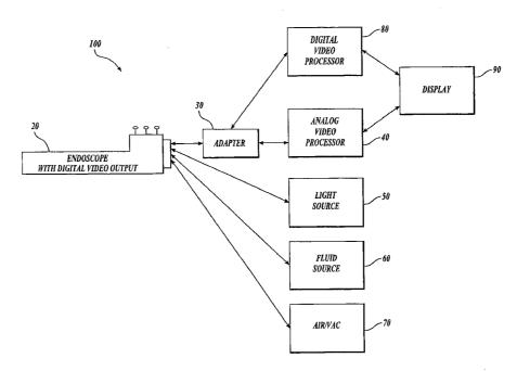
(57) Abstract: An adapter that allows digital imaging devices to be used with existing analog consoles. In one embodiment of the invention, an adaptor is provided that receives a digital video image signal from a medical device and converts the digital signal into an analog signal that can be displayed by an analog console. In another embodiment, the invention provides a method for converting a digital video signal received from a medical imaging device into a standardized analog video format.
