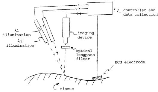
(57) Abstract: The present invention provides various methods/systems of optical imaging of subsurface anatomical structures and biomolecules utilizing red and infrared radiant energy. Also provided are various applications of such methods/systems in medical diagnosis and treatment.
