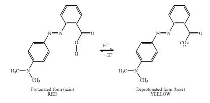
As a representative example, it is shown here that when the reaction involves Methyl Red, when it is placed on a white paper substrate, the colorless or first colored state (base form) provides a yellow state to the paper, while the colored or 45 second colored state (acid form) provides a red image to the paper.
