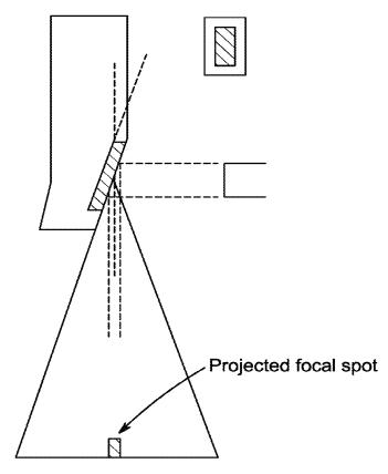
Poor field coverage Small effective focal spot Good power loading
