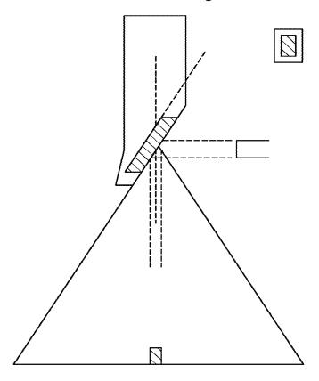
Good field coverage Small effective focal spot Poor power loading
