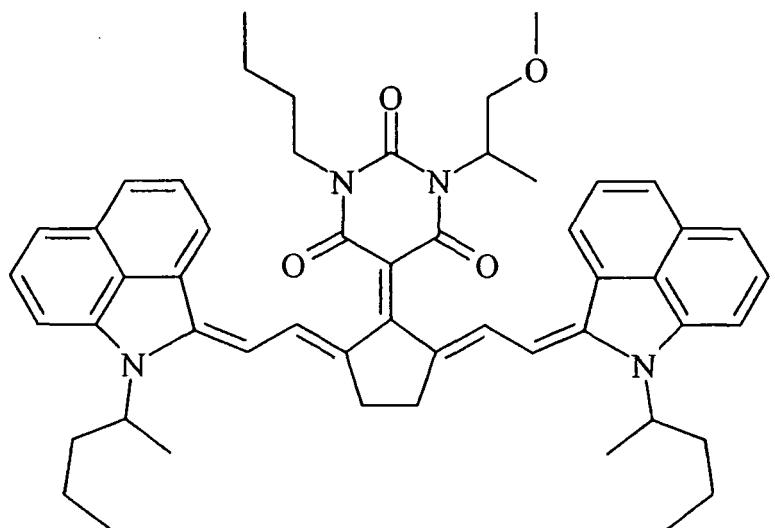
20 The infrared dye IR-1 has an absorption maximum  $\lambda_{\text{max}}$  of 1052 nm making it very suitable for a Nd-YAG laser having an emission wavelength of 1064 nm.
