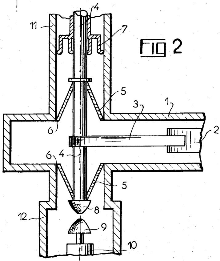
**SYSTEM FOR FEEDING ELECTROMAGNETIC ENERGY INTO A CYCLOTRON AND A CYCLOTRON INCORPORATING SUCH SYSTEM**
