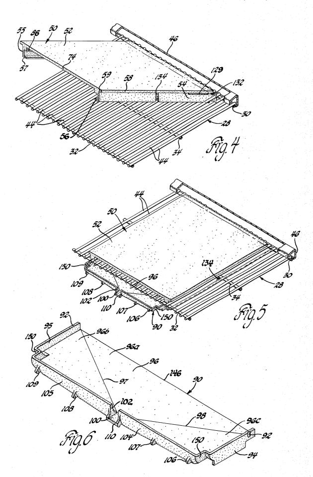
REFRIGERATOR RECEPTACLE SUPPORT AND ADJUSTABLE AIR DEFLECTOR-DRIP TRAY
