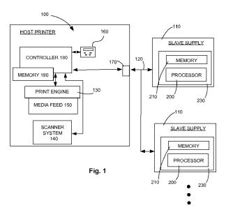
(57) Abstract: A new system and method for communicating between a host device and one or more slave devices are presented. The system provides data error checking and correcting, data encryption, and robust slave address sequencing using a portion of a session key. The data encryption uses a second portion of the session key, which changes for each power cycle.
