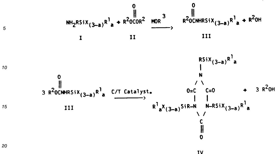
\*=Cracking and/or Trimerization Catalyst
