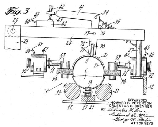
MECHANISM FOR ARRANGING SIDE SEAMS OF CANS
