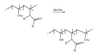
**[0108]** Following the hydrolytic procedure of Example P3, the copolymer of Example P3 (212 g) is further hydrolyzed to yield the title copolymer (200 g) as a white solid having a molecular weight of 195,000 as determined by gel permeation chromatography (GPC). An
