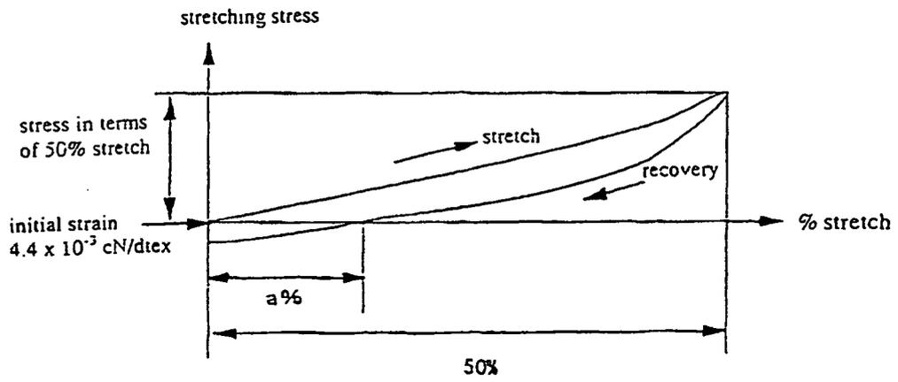
Figure 1: Stress-strain hysteresis curve diagram
