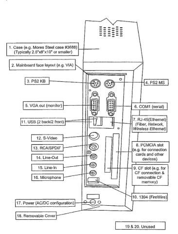
(57) Abstract: The present invention is directed generally to a smart modem device for vehicular and roadside applications for remote data collection and transmission to a central data collection and processing facility. The modem includes a number of sets of connection managers and monitors for performing specified tasks with respect to connections with various networks. Each set of connection managers and monitors is different and corresponds to a selected card type and/or network service.
