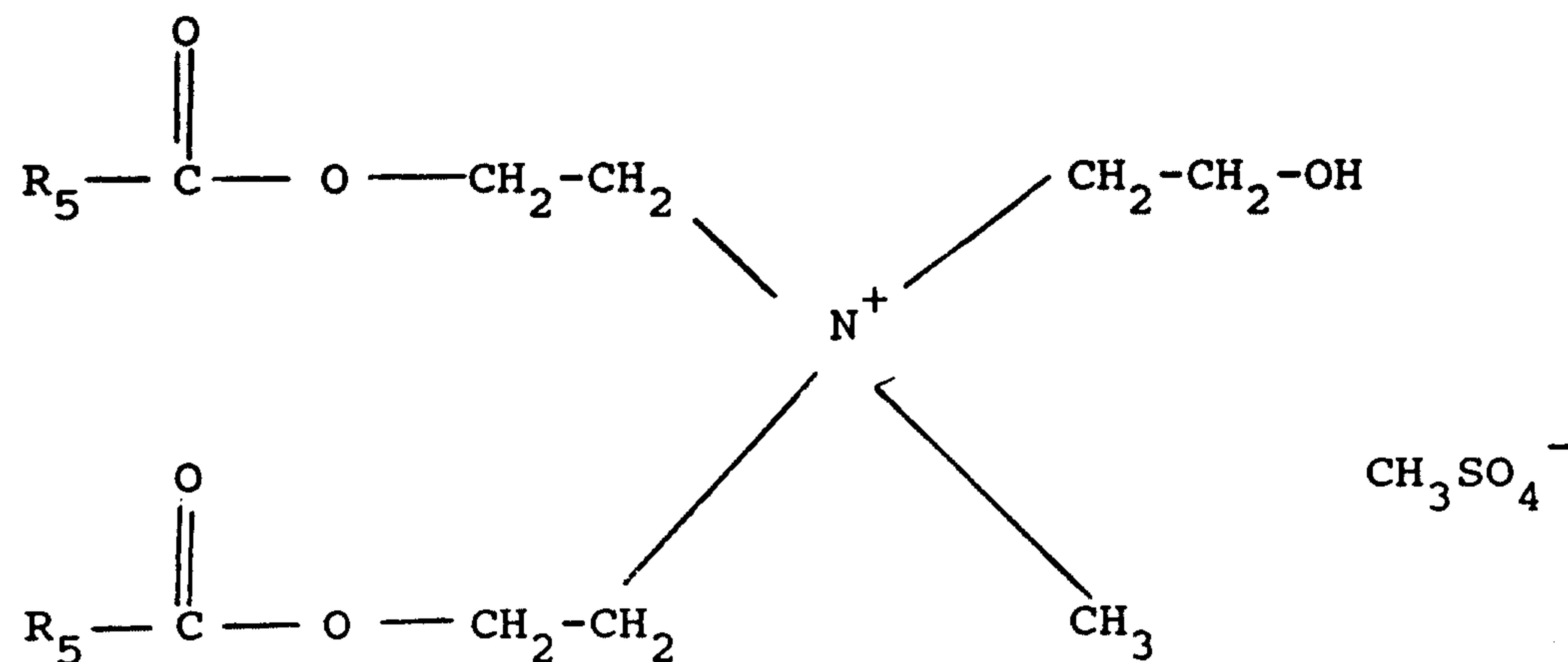
$R_5$  being tallow, which is available from Stepan under the trademark Stepantex VRH 90,
