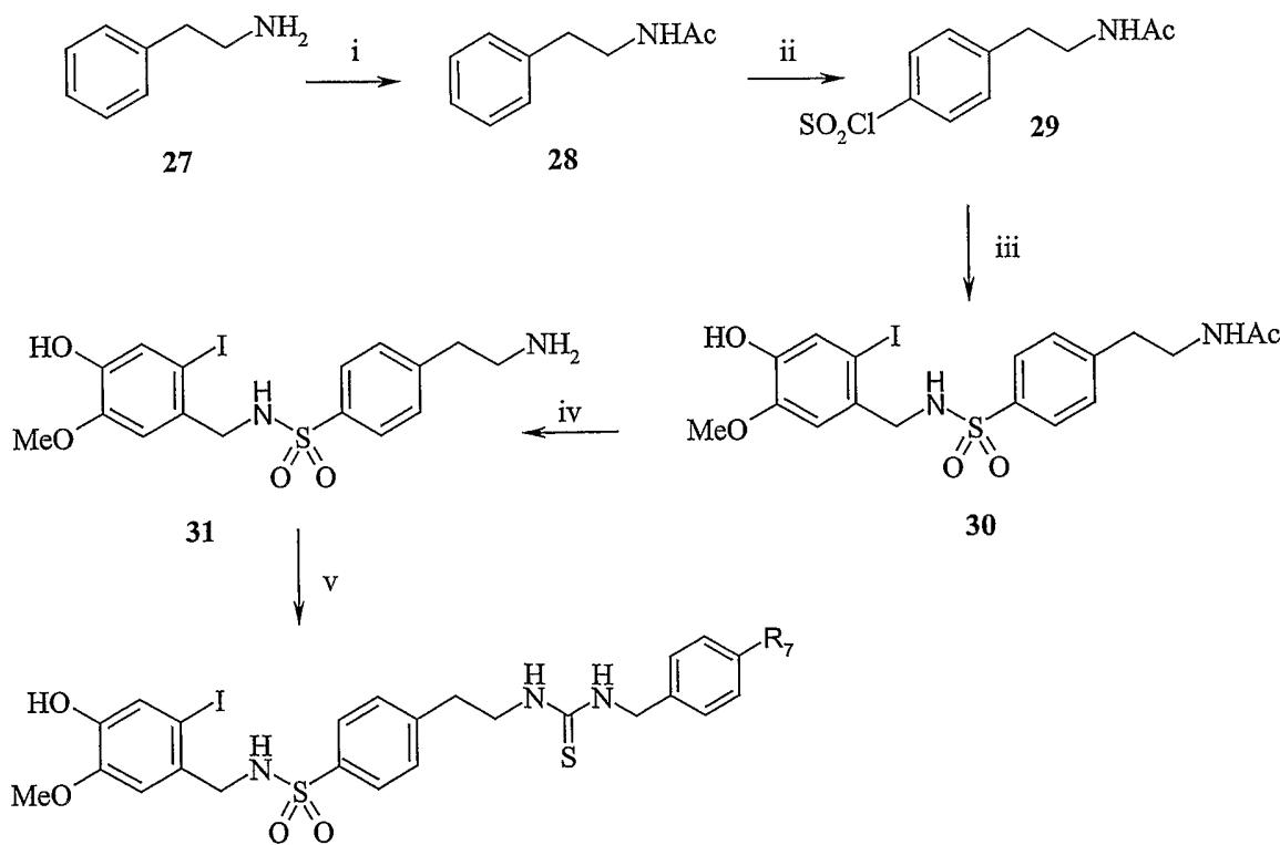
Reagents: (i) Acetic anhydride, (ii) chlorosulfonic acid, 0°C; (iii) 2-*ido*(chloro, bromo)-5-methoxy-4-hydroxy benzylamine hydrochloride, dioxane; (iv) aq. 20% NaOH; (v) 4-*tert*-butylbenzyl isothiocyanate or 4-trifluoromethylbenzyl isothiocyanate, ethanol, rfx.
