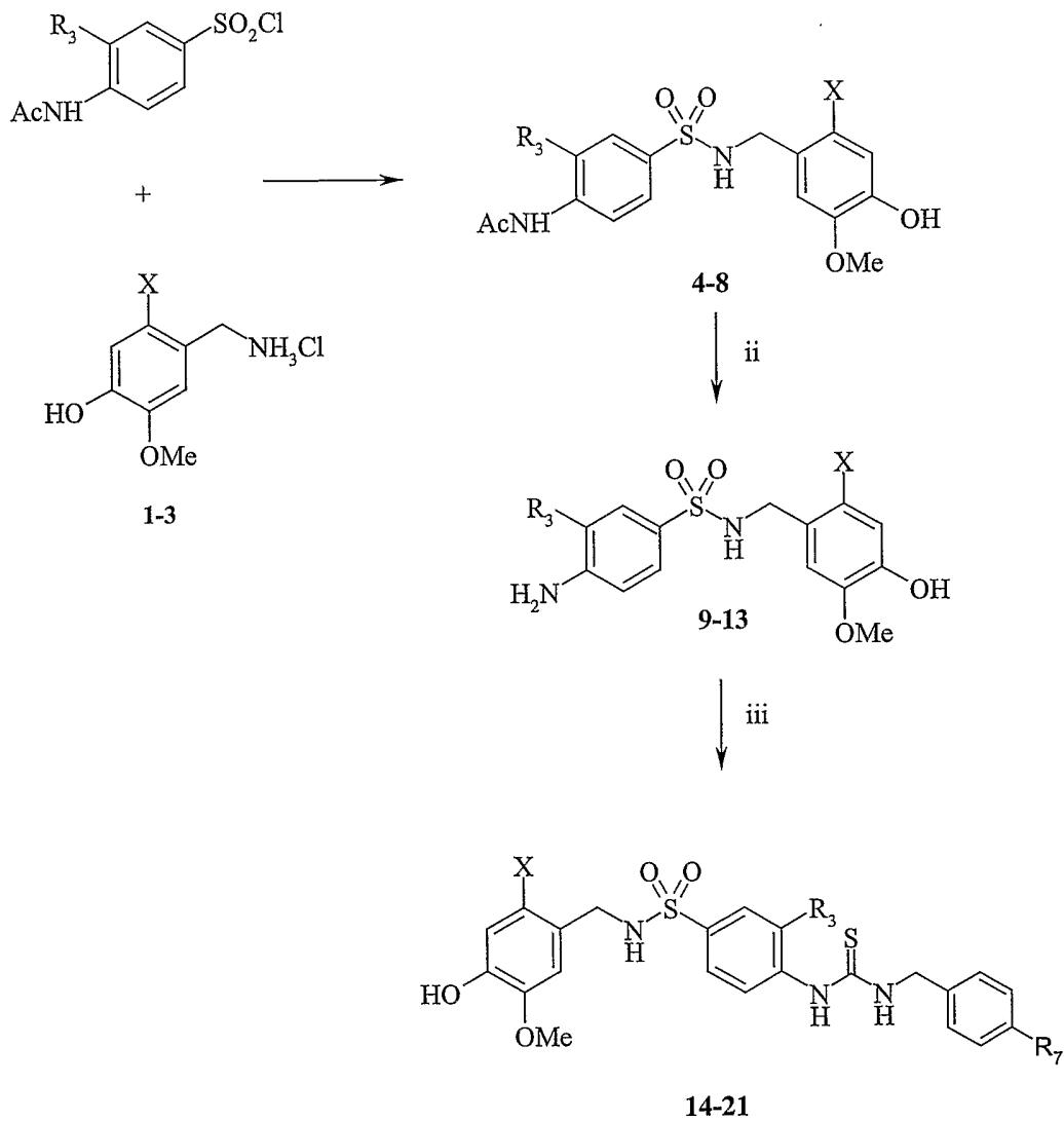
Reagents: (i) Dioxane, TEA, 80°C; (ii) aq. 20% HCl, dioxane; (iii) 4-5 *tert*-butylbenzyl isothiocyanate or 4-trifluoromethylbenzyl isothiocyanate, ethanol, rfx.
