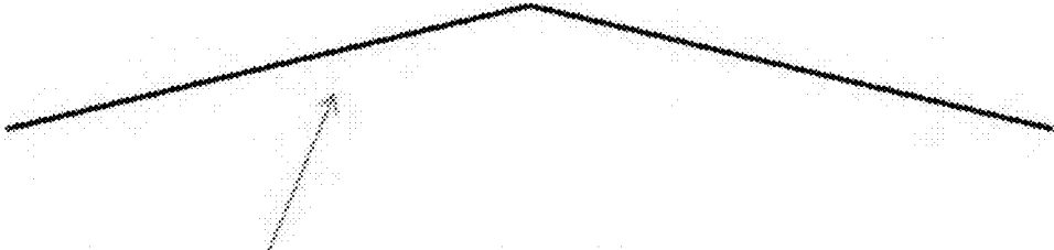
Side view of burner plate that is sloped so materials can roll or drain off
